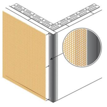
After 24 hours of drying, apply the final layer of glue on the hardened glue applied in this way, which is used for the final smoothing of the facade surface. After straightening, the mesh must not be visible. The position of the mesh in the finished reinforcing layer should be about 1/3 of the thickness of the layer on the side of the upper surface. The total thickness of the entire reinforcement-finish layer of glue should be 3-4 mm.
