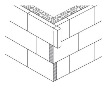
Glue the panels tightly together so that the glue does not reach the contact surfaces between the two EPS panels. Any cracks should be filled with pieces of EPS panel, or with lowexpansion pur foam for this purpose, BK-PUR EPS Kleber Gun, and never with glue.
