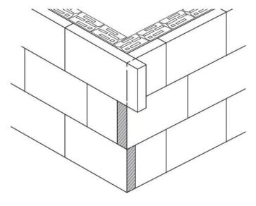
Glue the panels tightly together so that the glue does not reach the contact surfaces between the two EPS GRAFIT panels. Any cracks should be filled with pieces of EPS GRAFIT panel, or low-expanding PU foam for this purpose \_BK-PUR EPS Kleber Gun, and never with glue.
