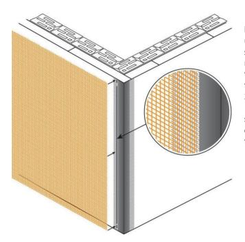
After 24 hours of drying, it is neccesary to apply the final layer of glue on the hardened glue applied in this way, which is used for the final smoothing of the facade surface. After straightening, the mesh must not be visible. The position of the mesh in the finished reinforcing layer should be about 1/3 of the thickness of the layer on the side of the upper surface. The total thickness of the entire reinforcement-finish layer of glue should be 3-4 mm.
